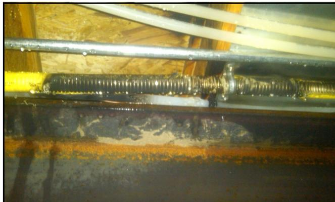
*CSST failure in 2010 shortly after a lightning strike. Fortunately, the plastic water pipe melted from the fire and extinguished the fire.*
